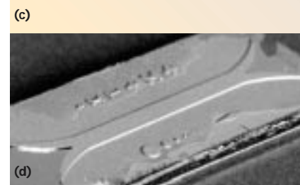
▲ Fig. 6 Fabricated micromachined K-band diplexer's (a) top and (b) bottom views and (c) frequency response, and (d) micromachined waveguide-based G-band (140 to 220 GHz) antenna.
